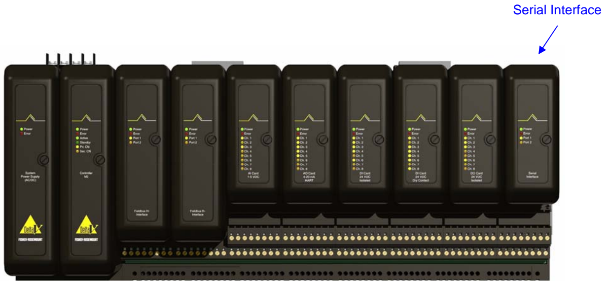
The DeltaV Serial Interface provides a connection between the DeltaV system and other devices.
